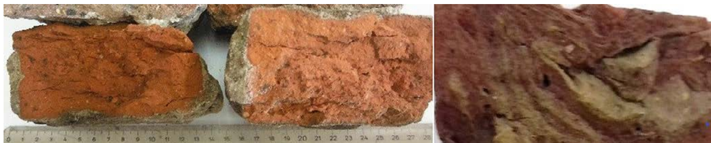
Figure 6 Typical appearance of the low temperature specimens. Left: rubbing bricks from the façade (B3). Right: B9 from the back wall. Photographs by Sara Pavia.
